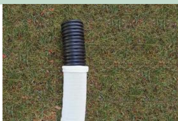
A sock-covered pipe usually costs more, but the benefits in terms of efficiency might outweigh the cost. All images courtesy of Ehsan Ghane.
